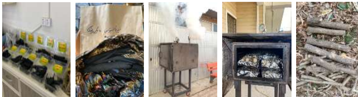
Figure (2): Stages of charcoal production from tree branches
