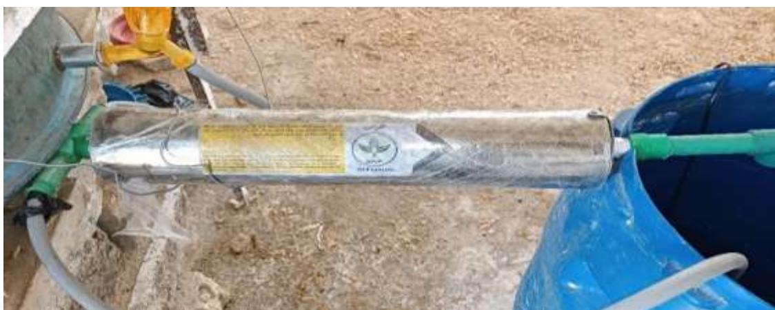
Figure (1). The water magnetizer device used in the experiment.
