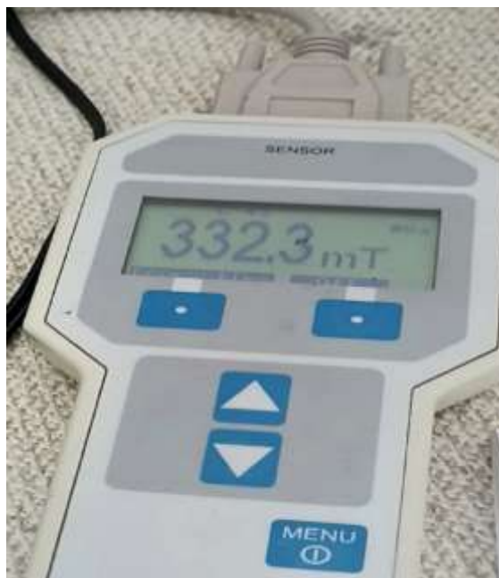
Figure (2). Measuring the intensity of the magnetic field of a magnetization device.
