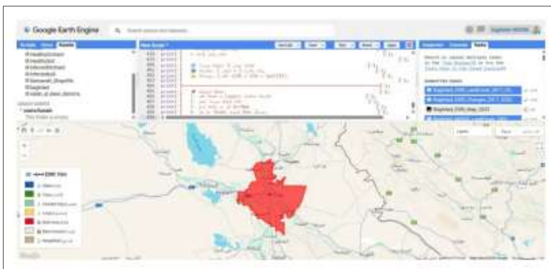
Figure 3. Google Earth Engine Code Editor environment showing the implementation of the processing workflow, including loading the Baghdad Province boundary, filtering the ESRI 10 m land-cover Image Collection, and executing server-side area calculations.
